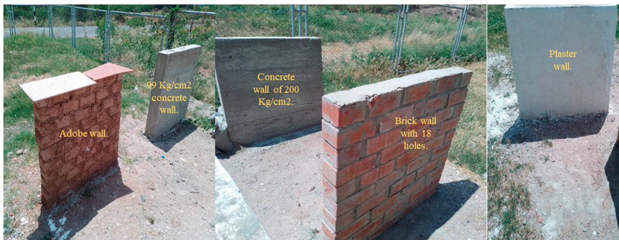
Figure 14. Specimens of different construction materials. Note: the specimens were constructed of adobe, brick, plaster, concrete and fine sand. Tests were conducted in open air “on specimens” one after the other, and this did not affect the results obtained because it was free from interference.
